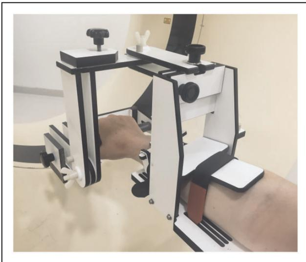
**Figure 2.** The participant lies in prone position with the hand enclosing a rod. This rod can be repositioned to place the wrist in the centre of rotation. The custom-made positioning device allows active wrist motion along the flexion–extension and radioulnar deviation motion axes.
